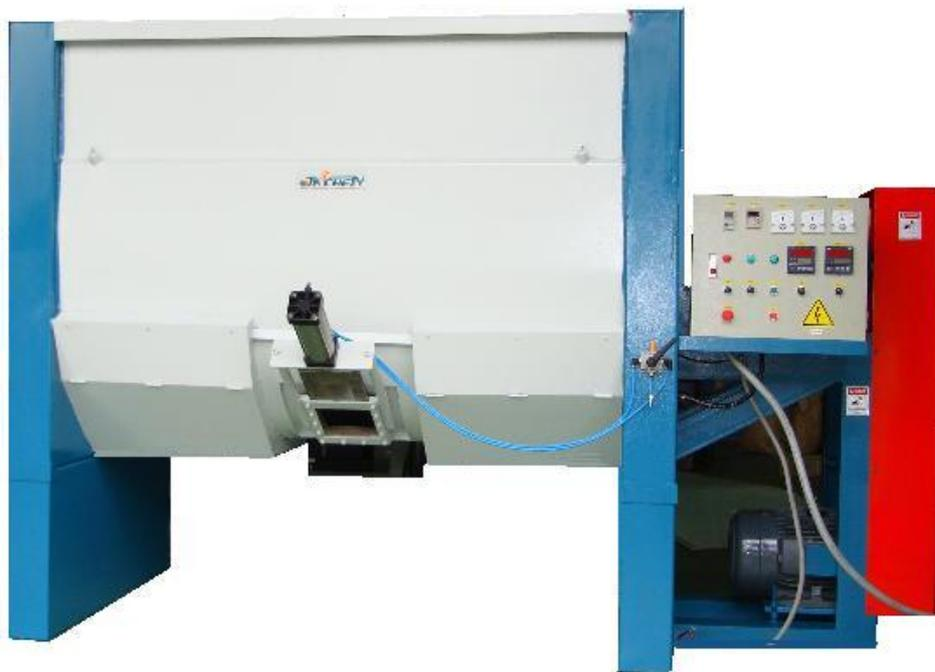
The newest mixer/composter specializes in mixing organic fertilizer & additive bacteria. It is able to put in kitchen wastes, vegetables, dead chickens, chicken excrements and so on for completely mixing, also to put in bacteria for high-speed fermentation. The specifications are easy installation and operation, time and labor-power saving. Moreover, the machine body is all made of stainless steel SUS304 for easy cleansing.
